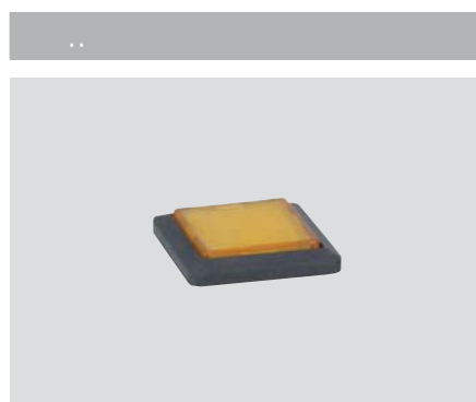
Signalling device With concave button Illuminated surface 19 x 19 mm 1 NO contact on DO A/ Slave Lamp replacement from front Available in 5 different colours Prints on device on request Ordering suffix, refer to table below
