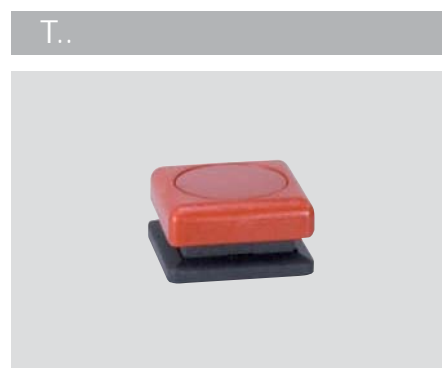
ushroom-shaped pushbutton Contact surface 25 x 25 mm with rounded sides Not latching 2 NO contacts or 1 NO/1 NC contact Available in 6 different colours Prints on device on request Ordering suffix, refer to table below
