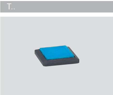
Illuminated pushbutton with concave button Contact surface 19 x 19 mm 2 NO contacts or 1 NO/1 NC contact Lamp replacement from front Available in 5 different colours Prints on device on request Ordering suffix, refer to table below
