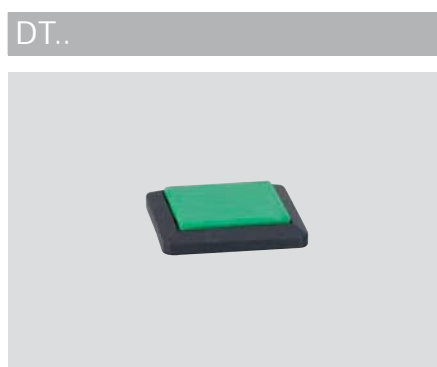
ushbutton With concave button Contact surface 19 x 19 mm 2 NO contacts or 1 NO/1 NC contact Available in 6 different colours Prints on device on request Ordering suffix, refer to table below
